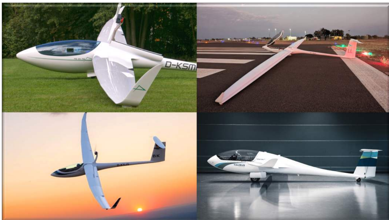
Leading edge electric propulsion technologies now incorporated in gliders and sailplanes in Australia: Clockwise from top left - Schleicher AS 34 ME, Diana FES, Pipistrel Taurus Electro, Jonker JS3 RES.
